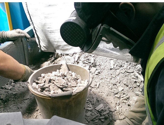
Our sampling facility consists of sieving, hammer-mill crushing and a paddle blender. This process mirrors that of the end user of the catalysts.
